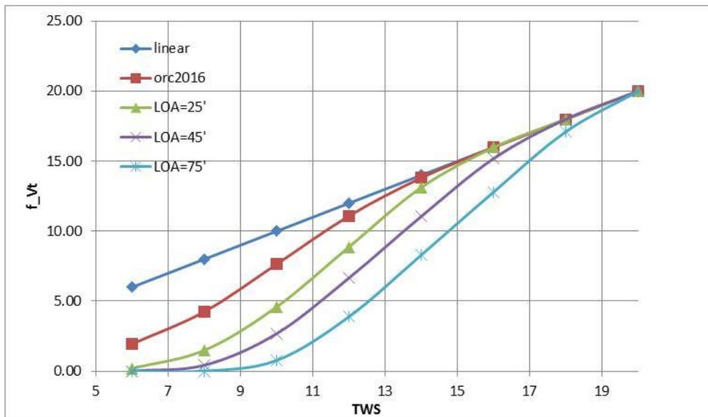
The above plot shows how the energy curve has been corrected for boats with LOA=25', 45', and 75'.
